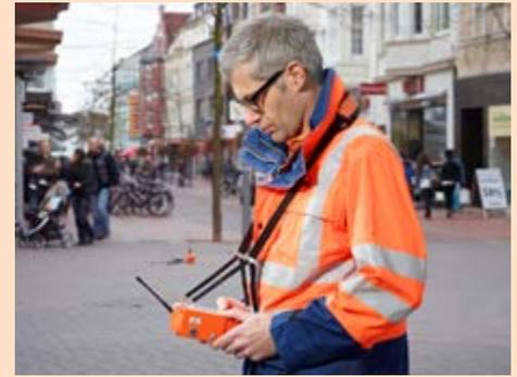
Figure 3: Pinpointing the leak with a correlator
